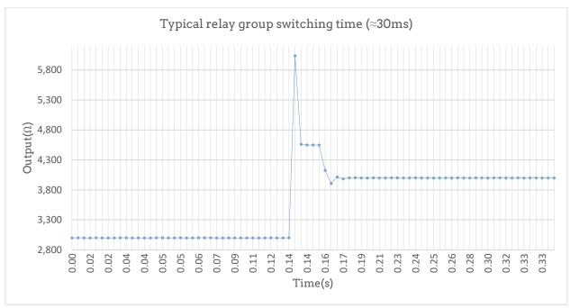
Above: Typical relay group switching time. The example is monitoring the process of switching from  $3k\Omega$  to  $4k\Omega$ , with the measurement mode 2-wire and the configuration NPLC=0.05.
