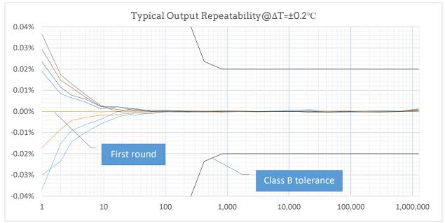
Above: Repeatability is based on the results of 8 consecutive rounds of testing of the same sample at room temperature (fluctuation range of about  $\pm 0.2^{\circ}$ C). Errors are based on comparison with the results of the first round.
